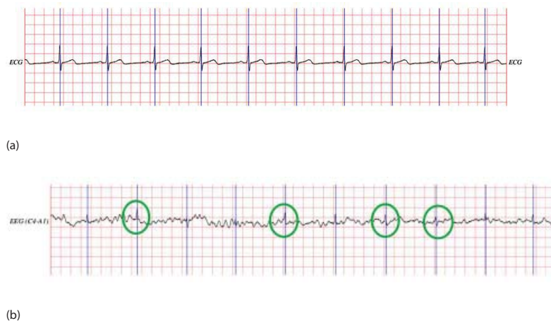
Figure 5: MIT-BIH dataset (a) ECG signal and (b) EEG signal with ECG noise [14].
